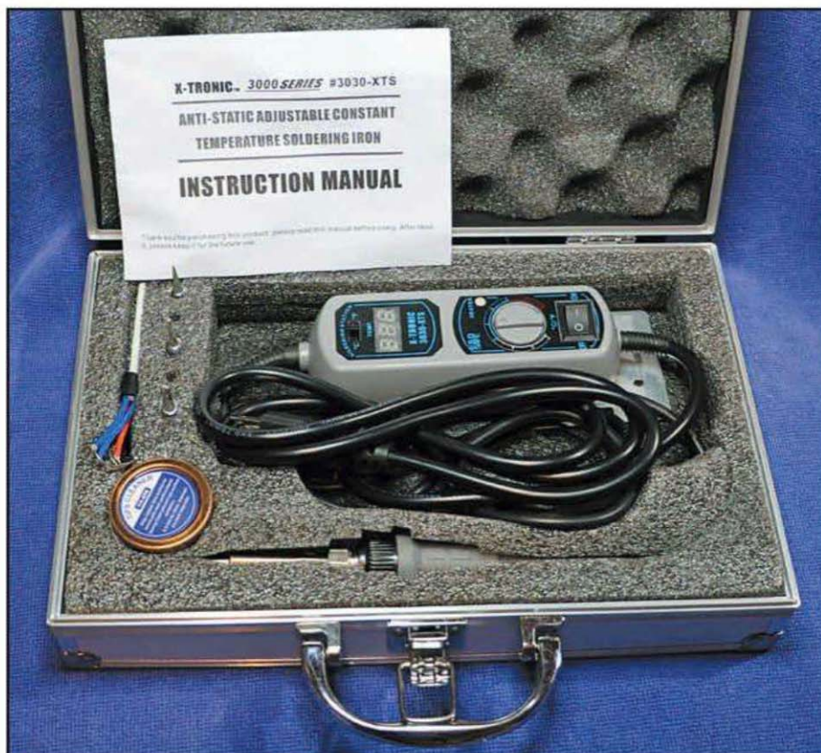
X-Tronic 3030 Travel soldering kit, complete with three different spare tips and a spare heating element.
