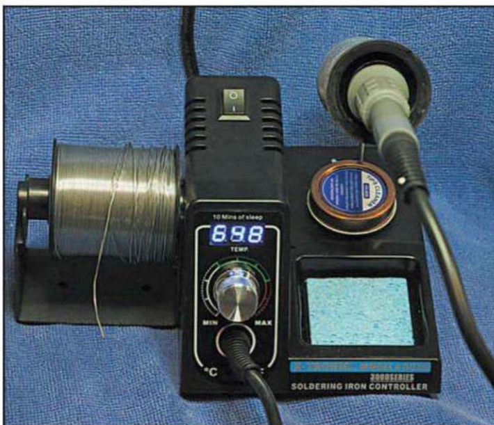
X-Tronic 3020 Soldering station warming up. Two different tip cleaners are included as is the solder roll holder, which attaches to the left side.
