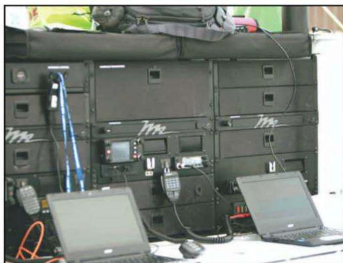
A Ham-Pod ready for use. The PC on the left is running DRATS and the one on the right is running FLDIGI.
