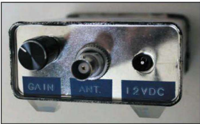
Photo C. The bottom of the Band-Aid box serves as the transceiver's rear panel. Note the rubber feet added for operating with the box placed horizontally.
