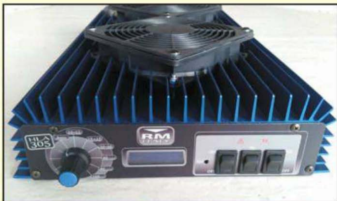
Photo D. RM Italy's newest amplifier, the HLA-305V, uses two large fans to quietly cool its sizable heat sink. It will produce up to 250 watts from QRP input for those times when 5 watts just can't get through reliably.
