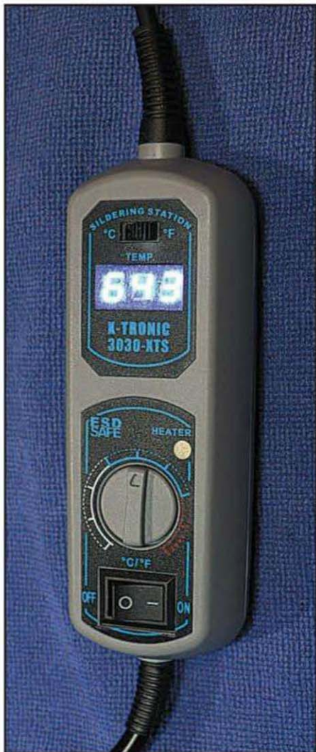
X-Tronic 3030 soldering iron in-line temperature controller.
