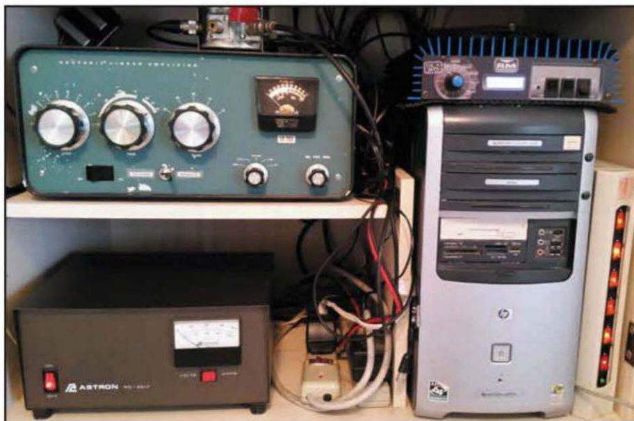
Photo C. Two RF amplifiers — the little RM Italy HLA-305 on top of the computer tower linked to the vintage Heathkit SB-200 on the left — provide me with the ultimate in QRP/QRO flexibility.
