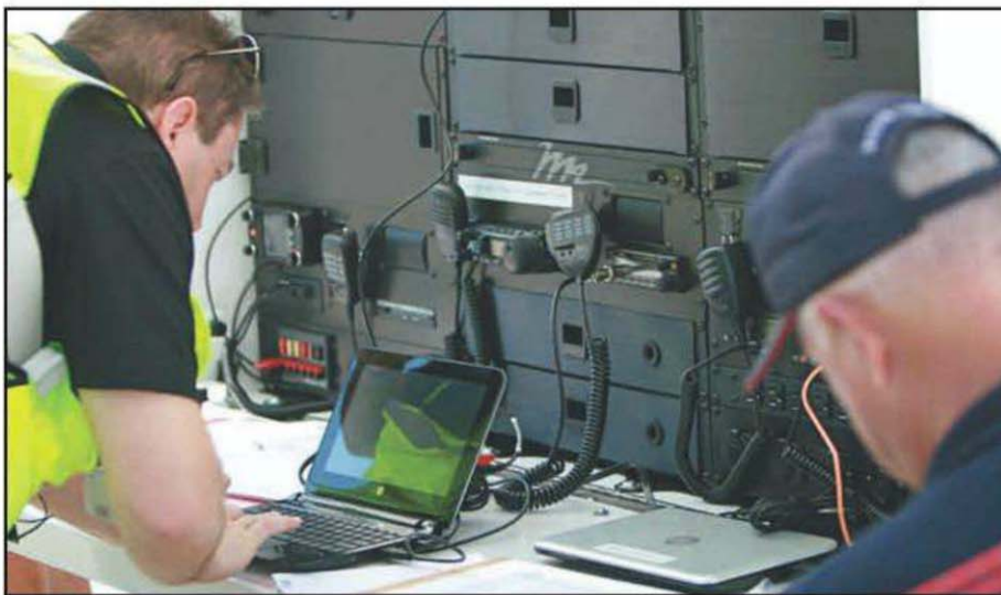
Author and ARRL SNJ Section Emergency Coordinator Tony Otlowski, W2WCC, sending NBEMS (Narrow Bandwidth Emergency Messaging System) traffic from a Ham-Pod at the air show.
