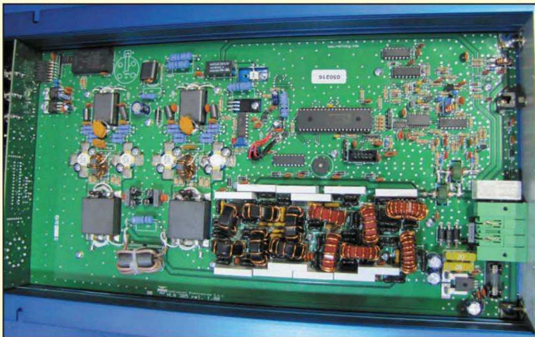
Photo E. A larger circuit board permits optimum component placement inside the HLA-305V. (Courtesy of RM Italy)
