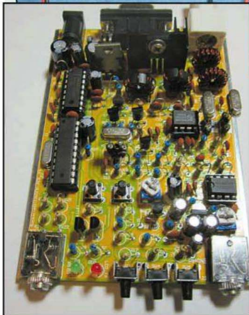
Photo A. Commonly-available QRP kits from China include copies or modified versions of well-known circuits designed in the U.S. and U.K. a generation ago, including the 49er, Frog Sounds, Pixie, and Rockmite. (Kit photos courtesy John Clements, KC9ON, < www.3rdPlanetSolar.com >)
